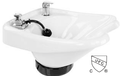
CB85-W SHALLOW PORCELAIN TILTING BOWL 19"W x 24"D x 9.5"H UPC APPROVED - FEATURING A TILT MECHANISM, 570 FAUCET, SPRAY HOSE, VACUUM BREAKER, DRAIN ASSEMBLY, HAIR STRAINER, AND FLEXIBLE TAIL STOCK (ALSO AVAILABLE IN BLACK AND NON-TILTING DECK-MOUNTED)
